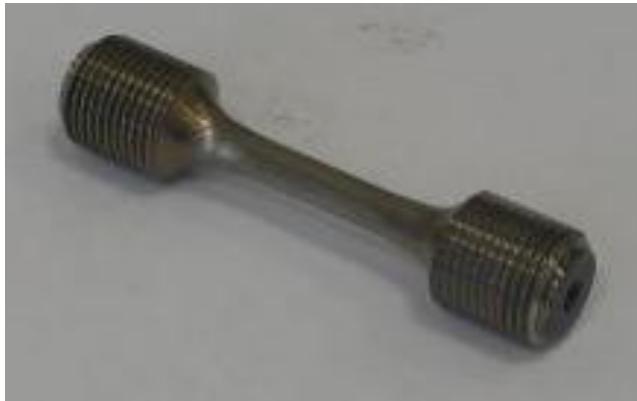
Figure 11 – Sample for short-time strength and low-cycle fatigue tests.
