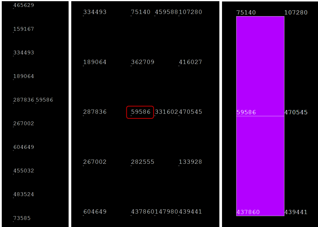
Figure 13.16 ANSYS crack front and adjacent nodes and contact elements.
