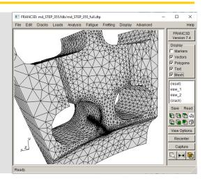
Version 8 supports these finite element analysis programs: ANSYS<sup>1</sup>, ABAQUS<sup>2</sup> and NASTRAN<sup>3</sup>. The fatigue life module supports combined low cycle (LC) and high cycle fatigue (HCF) loading. The crack insertion and meshing library allows symmetry surface cracks, embedded bi-material cracks, and cracks that cross bi -material interfaces. The Python interface is based on Python 3.9, but has been tested with older and newer versions of Python 3.
